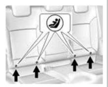
ISOFIX mounting brackets are marked by ② on the seat back.
