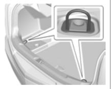
The cargo tie-downs can be used to secure small loads inside the boot.
