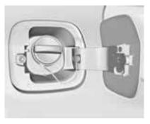
The cap is behind the fuel door on the passenger side of the vehicle. If equipped, the fuel door is locked when the vehicle doors are locked.
