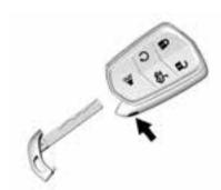
This key, inside the Remote Keyless Entry (RKE) transmitter, is used for the driver door and glove box.
