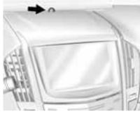
The solar sensor monitors the solar heat.
