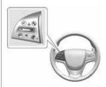
(S): Press to turn the system on and off. A white cruise control indicator appears in the instrument cluster when cruise is turned on.
