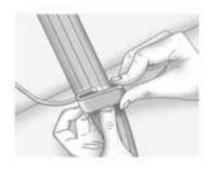
Place the guide over the belt, and insert the two edges of the belt into the slots of the guide.
