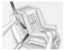
5. To tighten the belt, push down on the child restraint, pull the shoulder portion of the belt to tighten the lap portion of the belt, and feed the shoulder belt back into the retractor. When installing a forward-facing child restraint, it may be helpful to use your knee to push down on the child restraint as you tighten the belt.
