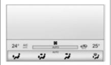
The climate control status screen appears briefly when the climate control buttons on the faceplate are adjusted. The air delivery mode can be adjusted on the climate control status screen.
