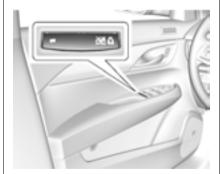
The rear door safety locks prevent passengers from opening the rear doors from inside the vehicle.
