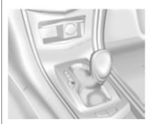
Vehicles with DSC may either use the shift lever or the tap shift controls on the back of the steering wheel (if equipped) to manually shift the automatic transmission.
