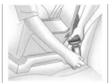
3. Push the latch plate into the buckle until it clicks. If the latch plate will not go fully into the buckle, check if the correct buckle is being used.
