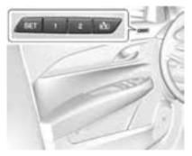
If equipped, the "1," "2," SET, and (Exit) buttons on the driver door are used to manually store and recall memory settings for the driver seat and outside mirrors.
