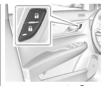
From the inside, press or or a. The indicator light in the switch will illuminate when locked. See *Power Door Locks on page 2-11*.
