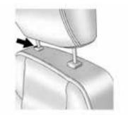
To lower the outboard head restraint, press the button, located on the top of the seatback, and push the head restraint down. Try to move the head restraint after the button is released to make sure that it is locked in place.
