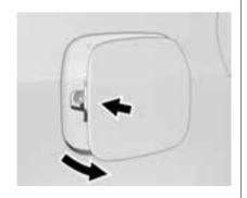
To open the fuel filler flap, push and release the rearward centre edge of the flap.
