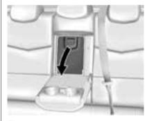
This vehicle may have a rear seat pass-through door in the centre of the rear seat backrest. Fold down the centre armrest and pull the latch to open the door.
