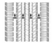
Tread wear indicators are one way to tell when it is time for new tyres. Tread wear indicators appear when the tyres have only 1.6 mm (1/16 in) or less of tread remaining. See *Tyre Inspection on page 10-44* and *Tyre Rotation on page 10-44*.
