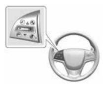
The Collision Alert control is on the steering wheel. Press to set the FCA timing to Far, Medium, Near, or on some vehicles, Off. The first button press shows the current setting on the DIC. Additional button presses will change this setting. The chosen setting will remain until it is changed and will affect the timing of both the Collision Alert and the Tailgating Alert features. The timing of both alerts will vary based on vehicle speed. The faster the vehicle speed, the farther away the
