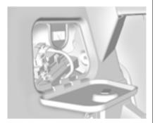
The rear compartment fuse block is behind a cover on the driver side of the rear compartment.
