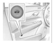
To open the boot, press from inside the vehicle or press twice quickly on the Remote Keyless Entry (RKE) transmitter, or press the touch pad on the rear of the boot above the number plate after unlocking all doors. See Remote Keyless Entry (RKE) System Operation on page 2-2 and Boot on page 2-13.
