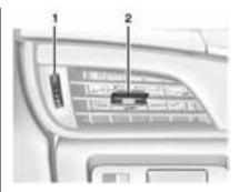
Move the slats (2) to change the direction of the airflow.
