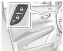
(Lock): Press to lock the doors. The indicator light in the switch will illuminate when activated.
