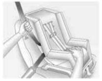
4. To tighten the belt, push down on the child restraint, pull the shoulder portion of the belt to tighten the lap portion of the belt, and feed the shoulder belt back into the retractor. When installing a forward-facing child restraint, it may be helpful to use your knee to push down on the child restraint as you tighten the belt.
