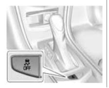
The button for TCS and StabiliTrak is on the centre console, behind the gear lever.
