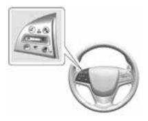
(On/Off): Press to turn the system on and off. A white cruise control indicator appears in the instrument cluster when cruise is turned on.
