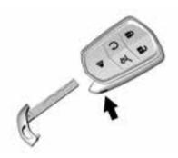
Press the button on the side of the transmitter near the bottom and pull the key out.
