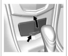
To access, press on the cover and release. There is an accessory power outlet inside. See *Power Outlets on page 5-6*.
